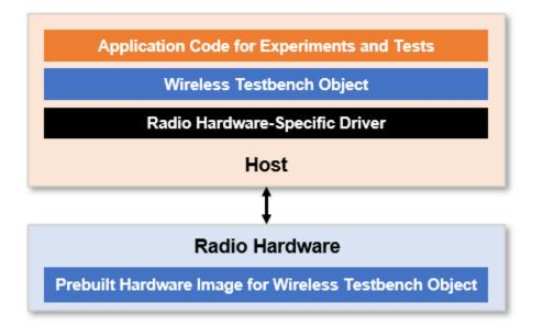
Using a Wireless Testbench object, you can configure the prebuilt hardware image to transmit, capture, or detect wireless signals and write your application code for experimenting and testing.
