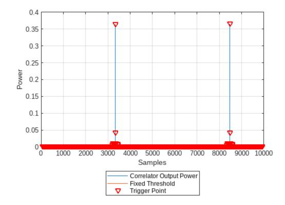
Choose a threshold value that is below any of the trigger point values. Plot the threshold information again and adjust the fixed threshold until the trigger points appear only on the correlator output peak. Run the plotThreshold function multiple times to see any sampling phase effects.
