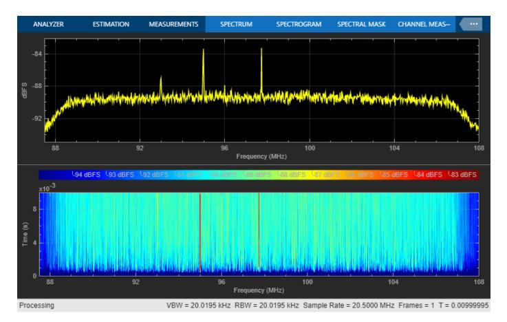
To call the capture function again and to update the spectrum analyzer by rerunning the current section, click **Capture and plot frequency spectrum**.
